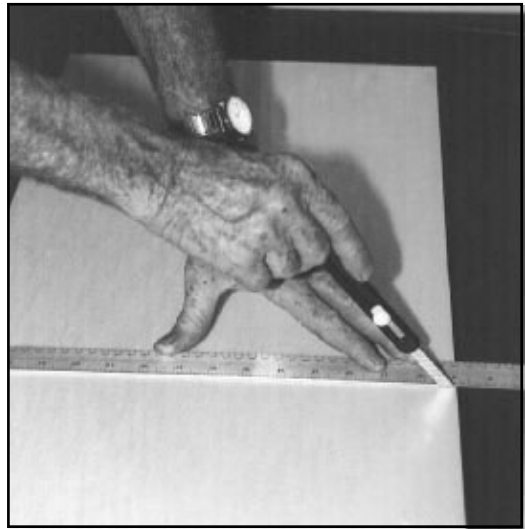
Figure 2. The foam panels are easily cut with a utility knife and straight edge. A bandsaw or tablesaw may also be used.
