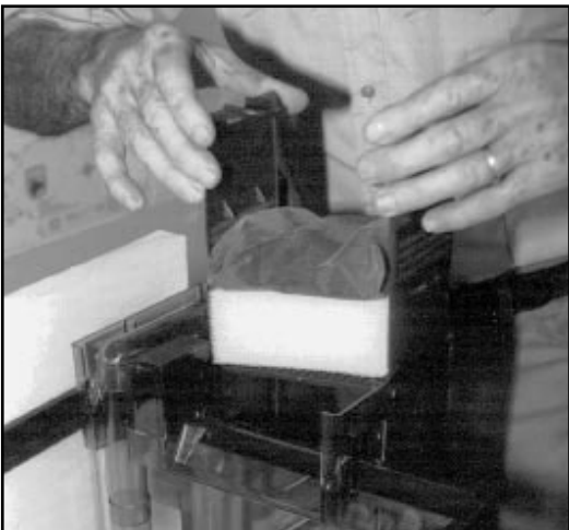
Figure 5. When placing filter elements into the filter basket, the foam element must be at the bottom.
