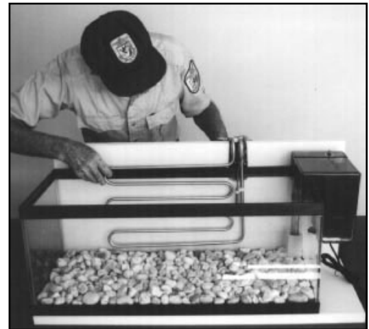
Figure 4. The chiller coil is lowered into the aquarium over the back styrofoam panel.
