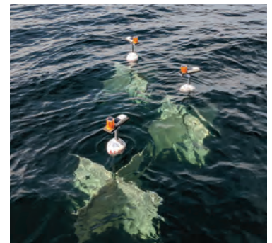
Ocean drift buoys used to research where lobster larvae may disperse as passive plankton in the Gulf of Maine region
